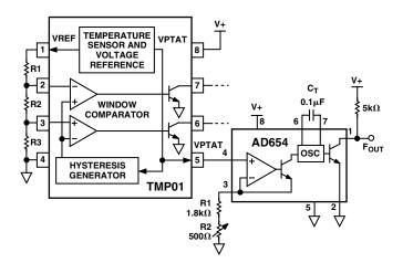
Figure 11. Temperature-to-Frequency Converter
