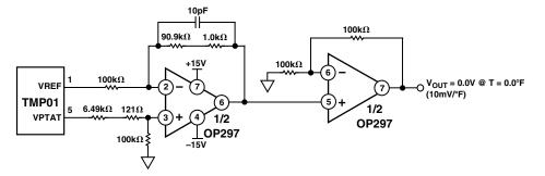
Figure 15. Translating 5 mV/K to 10 mV/°F
