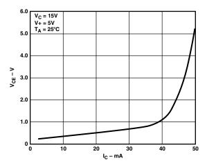
TPC 5. Open-Collector Output (OVER, UNDER) Saturation Voltage vs. Output Current
