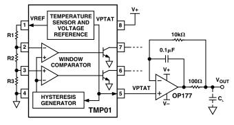
Figure 8. Buffer VPTAT to Handle Difficult Loads
