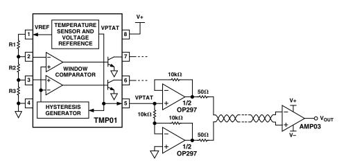
Figure 9. Send the Signal Differentially for Noise Immunity
