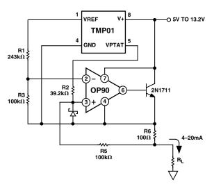
Figure 10. 4mA to 20 mA Current Loop
