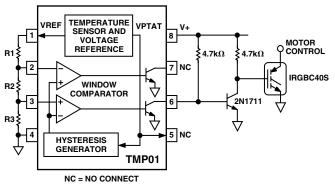
Figure 6d. Driving an IGBT
