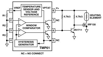
Figure 6c. Driving a N-Channel MOSFET
