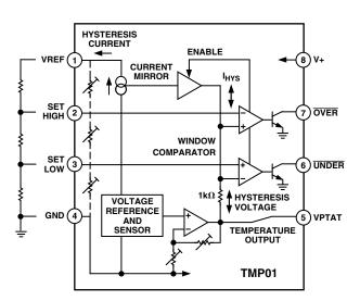
Figure 2. Detailed Block Diagram
