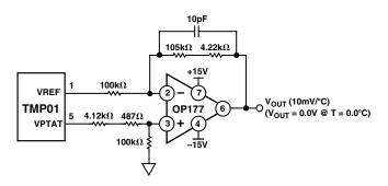
Figure 14. Translating 5 mV/K to 10 mV/°C
