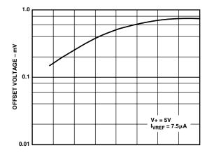
TPC 8. Set High, Set Low Input Offset Voltage vs. Temperature
