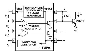
Figure 7a. An External Resistor Minimizes Self-Heating
