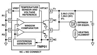
Figure 6b. Driving a P-Channel MOSFET
