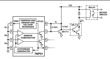
Figure 7c. Darlington Transistor Can Handle Large Currents
