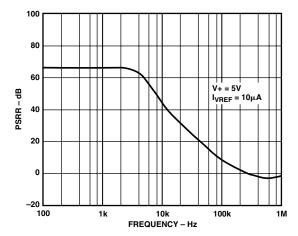
TPC 7. VREF Power Supply Rejection vs. Frequency
