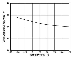
TPC 2. Minimum Supply Voltage vs. Temperature
