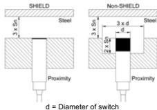
d = Diameter of switch Sn = Sensing distance
